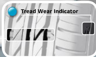
The legal limit of 1.6mm is reached when the tyre is worn to the level of the tread wear indicators in the main grooves.
